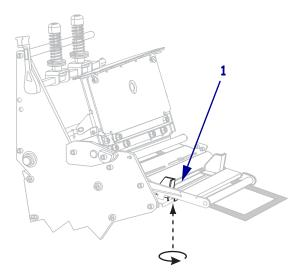
**11.** Push down the printhead assembly (**1**), and then rotate the printhead-open lever (**2**) clockwise until it locks into place.
